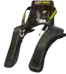
PRO HANS device. Lightweight carbon fibre PRO version. Equipped with sliding tethers and patented SlipStop Plus contact surface with retaining winglets. Weight around 520g. Available in medium only and 10 or 40 degrees.
